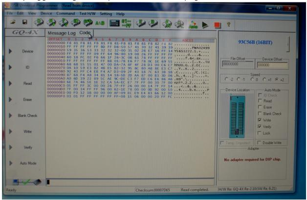
Note that when you read off the data, the bits will be swapped. To correct this, simply click on the icon at the top of the screen showing A-B. You will know that you have it right when you can read the VIN in the column headed ASCII. The VIN starts in the middle of the second line and ends in the first half of the third line. You may want to read your Boxster chip first so you will know the VIN you are looking for.
