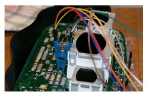
Here's a view of the SOIC clip attached to the circuit board. Once the clip is on the chip and the cable plugged in to the programmer you should select the chip type in the programmer software as a 93c56. Note that there are several choices for 93c56 chips in the
