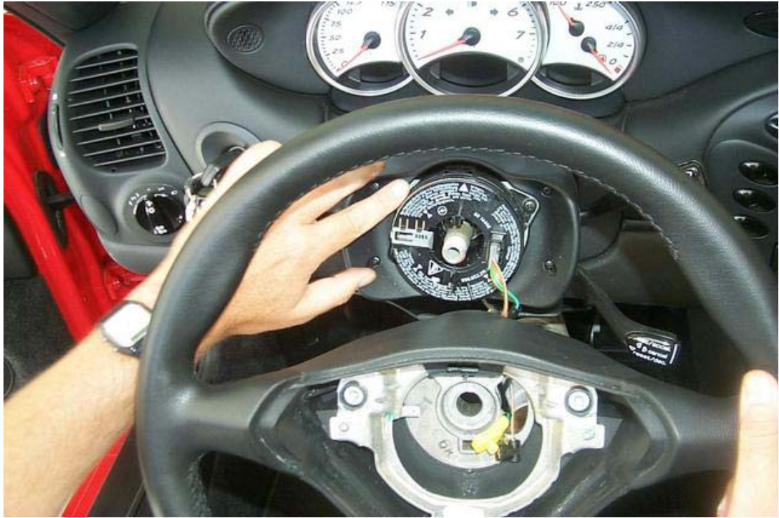
12 remove steering wheel – carefully feed wires through wheel
