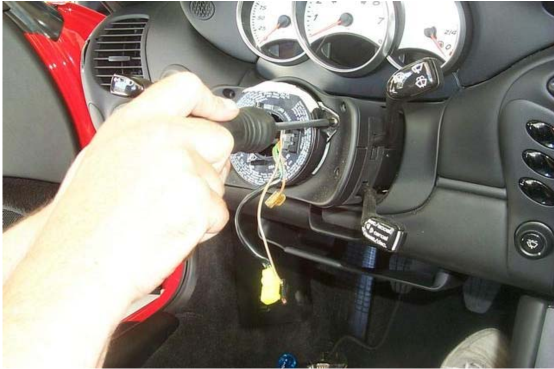
16 remove two Philips screws on airbag spring unit
