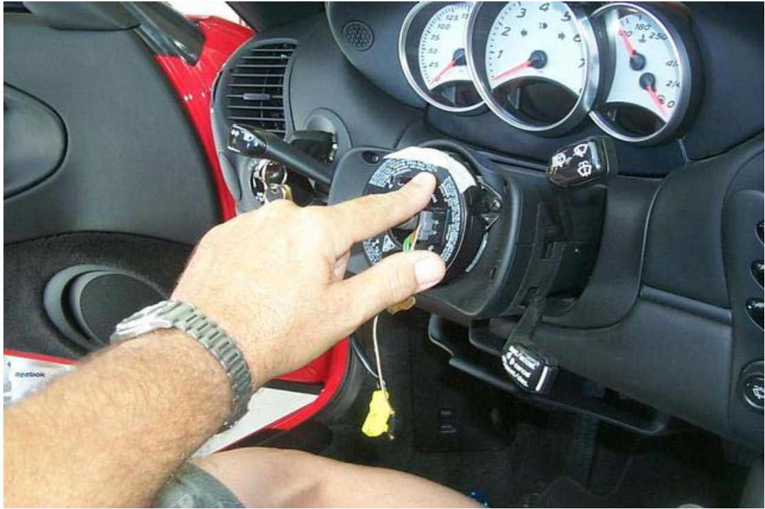
14 tape airbag spring unit so it doesn't rotate
