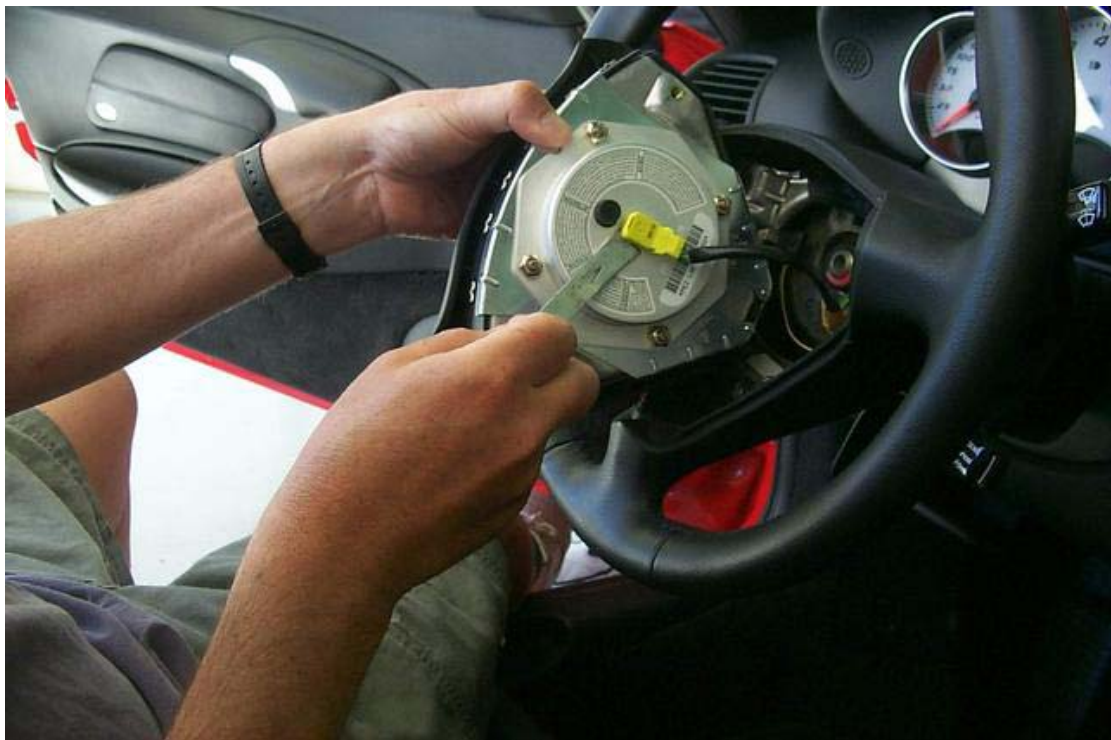
05 here's airbag connector being removed
