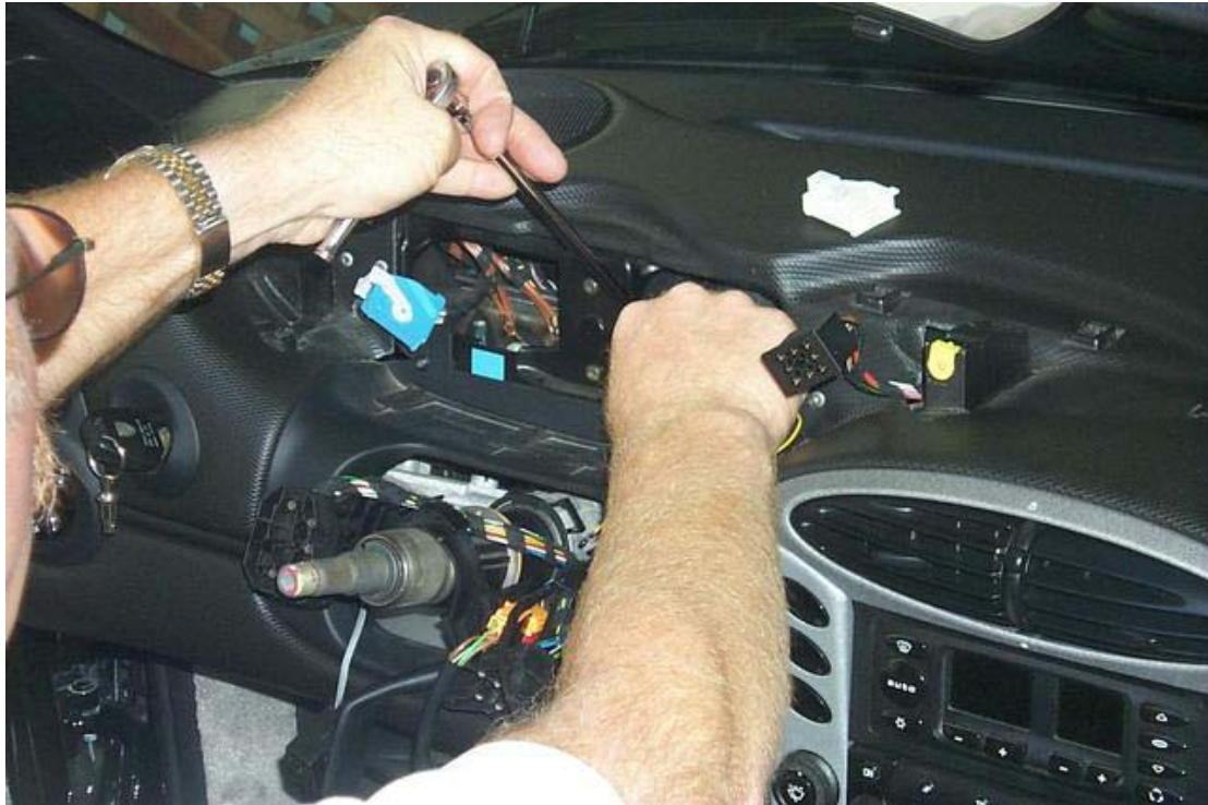
37 tightening up the nut holding the ground lug on
