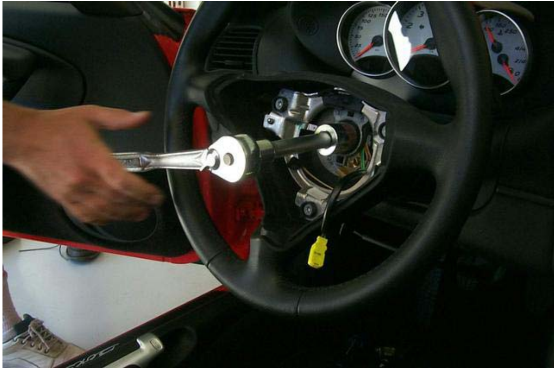
08 remove steering wheel nut
