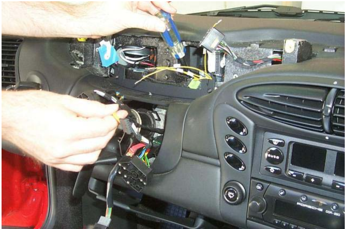
34 follow instructions for connection of wires to connectors and wire routing – as shown
