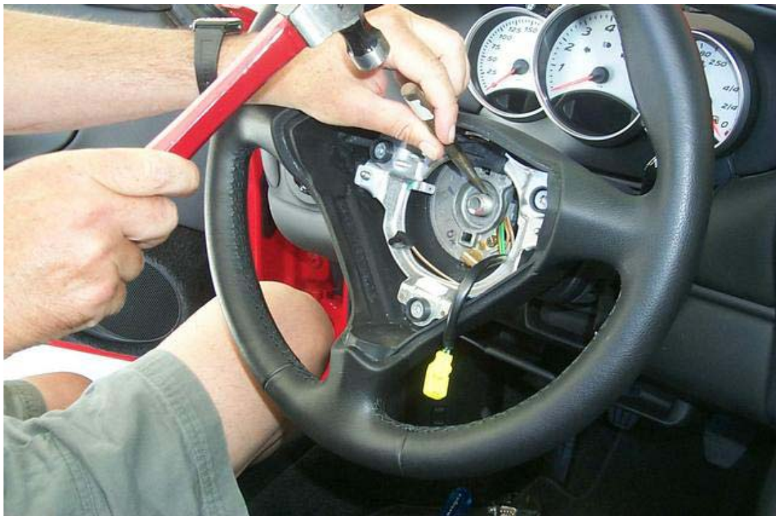
09 use punch to mark both steering wheel and bolt for matching location when reinstalling
