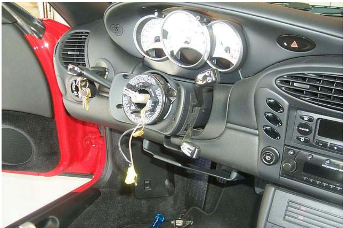
13 steering wheel removed, air bag spring unit shown
