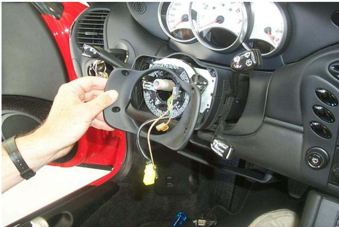
17 remove steering column housing fascia piece
