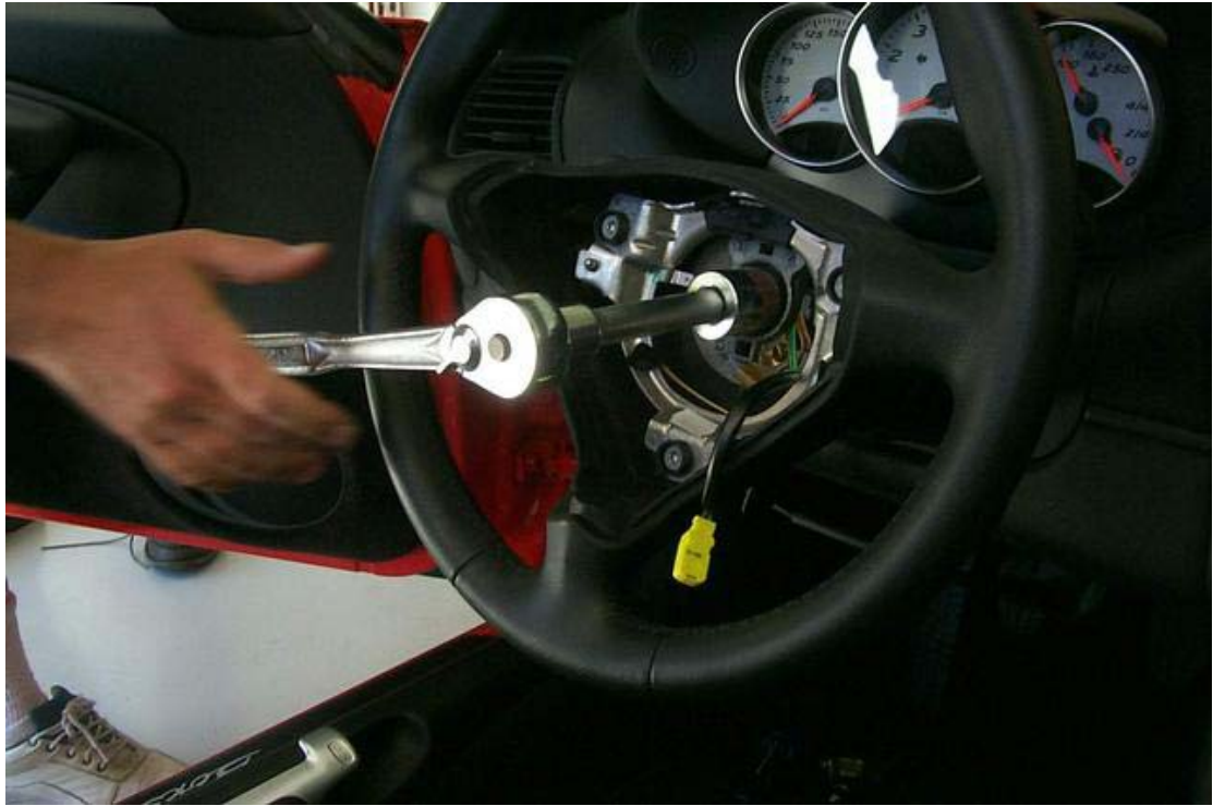
49 tighten steering wheel nut down - very little torque is needed! (just about hand tight - line up marks on nut and column)
