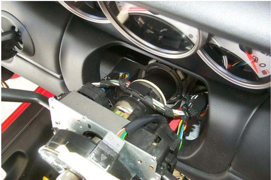
23 view from top of steering column housing removed
