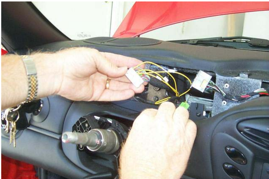
36 here is a view of the connector with the wiring harness wires installed
