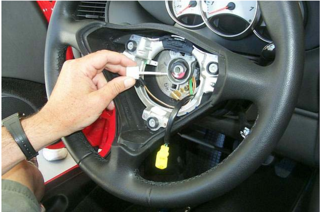
06 use white-out to mark location of steering wheel - mark both nut & center bolt together
