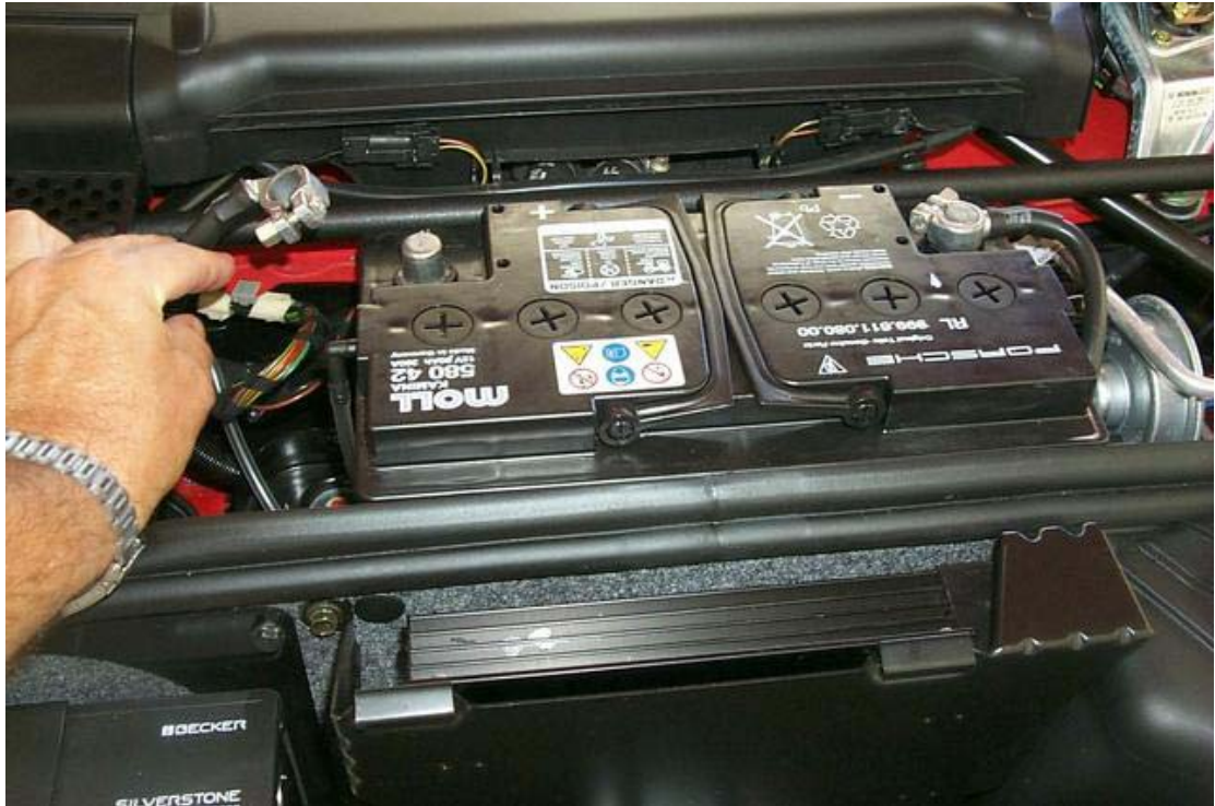
55 re-connect battery - typically you'd disconnect or re-connect the negative ground (not positive as shown)
