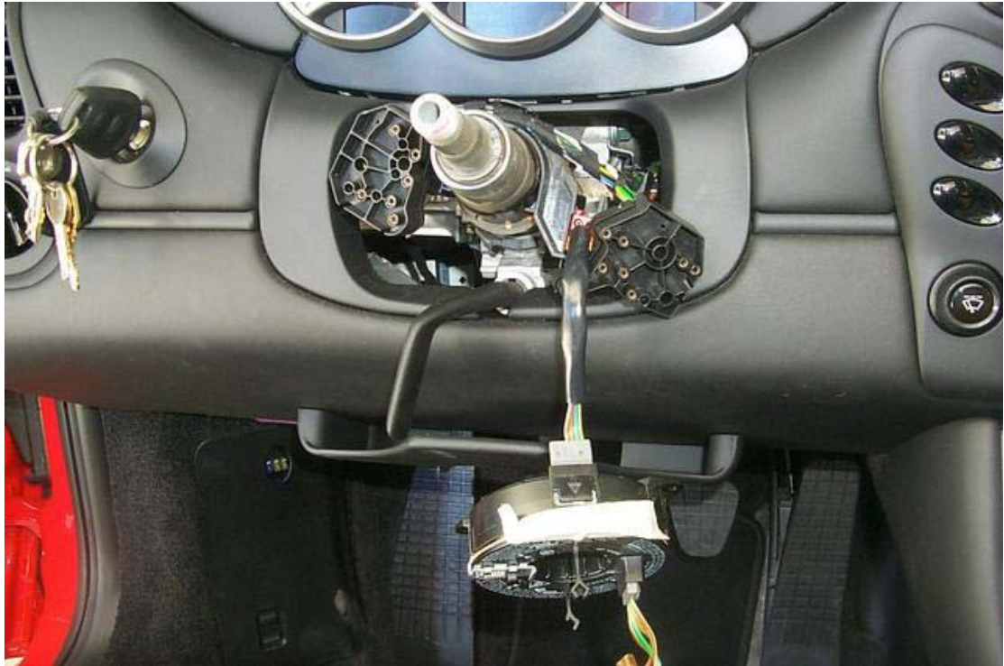
30 close up of steering wheel column area – note steering wheel fore-aft adjustment level position
