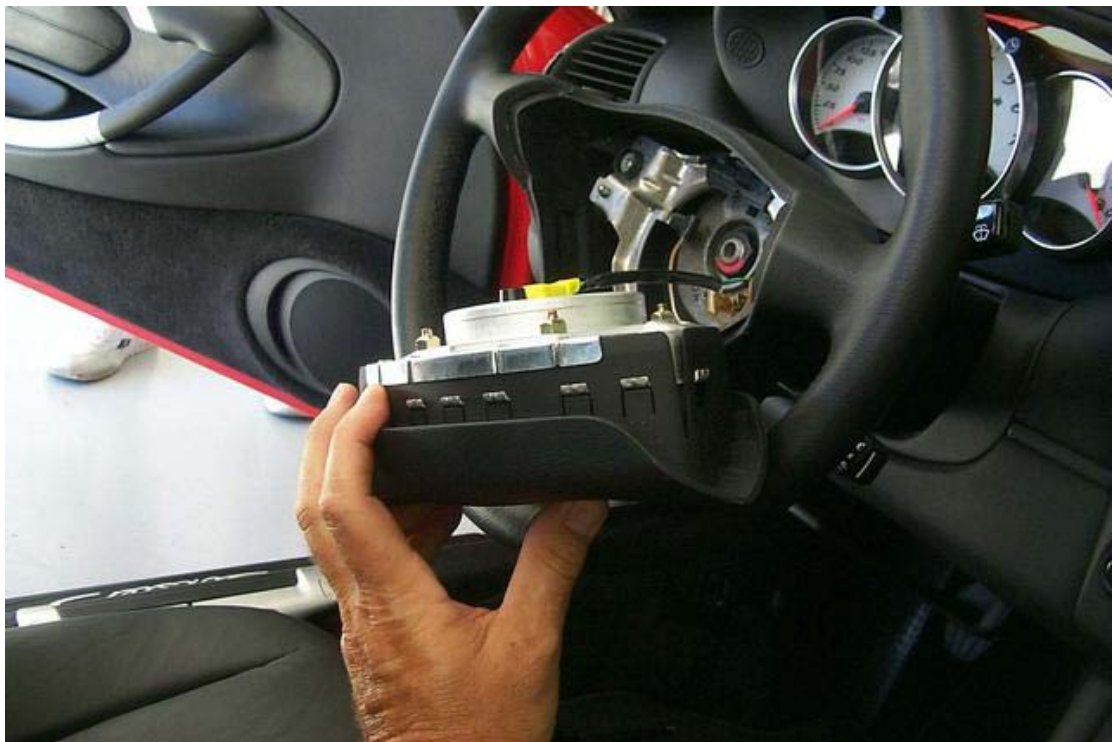
50 reinstall air bag connection - yellow plug presses on to connector
