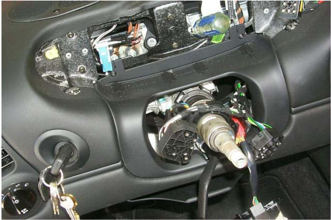
33 instrument pod is removed by lifting up on it – here socket screwdriver is loosening the ground lug for wiring harness
