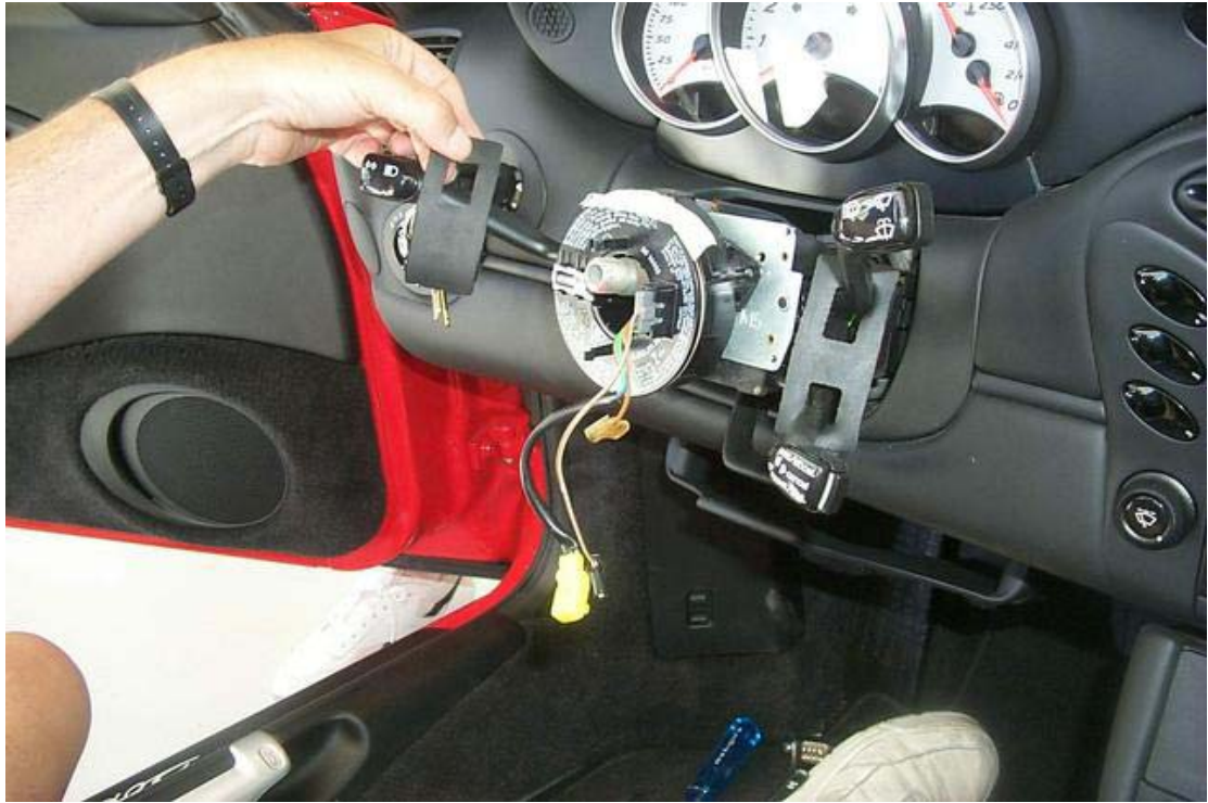
22 remove black rubber gaskets on each side – note larger hole goes on for stalks that have largest adjustment range
