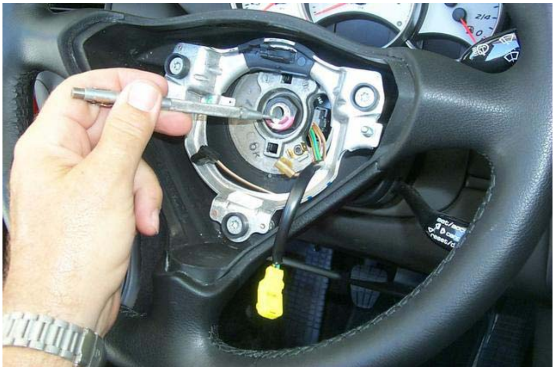
07 scribe white-out to note exact location of steering wheel for re-installation later
