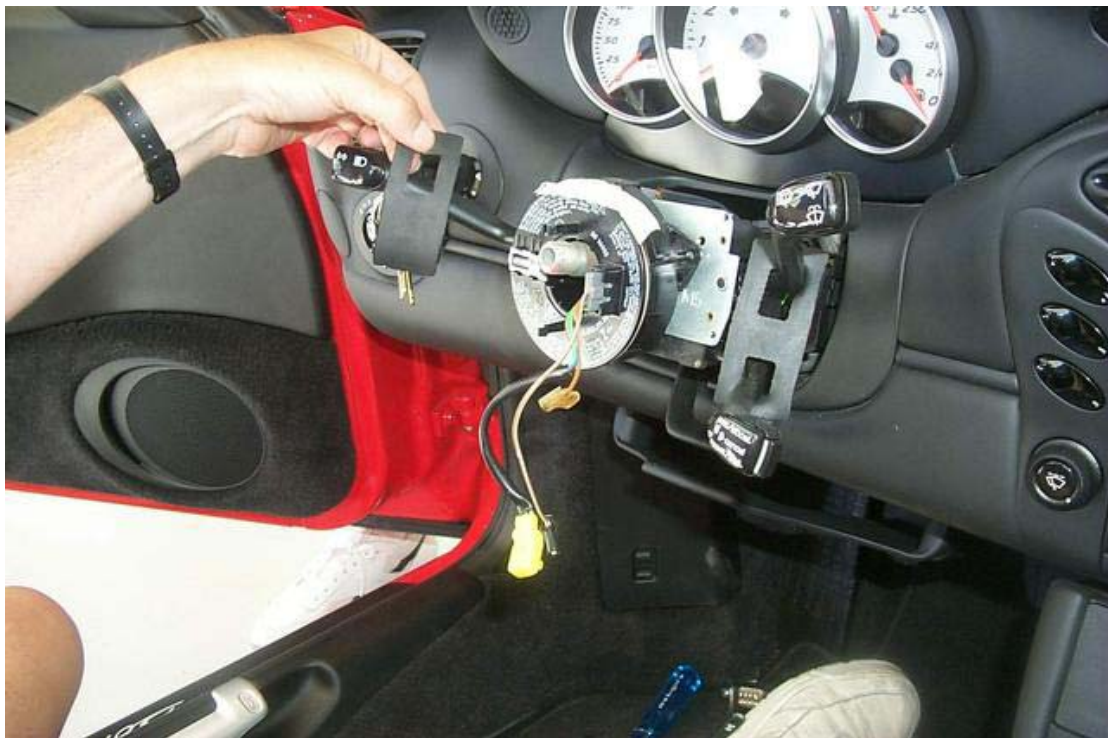
38 install 4-stalk assembly (3-Stalk shown here) & put on black rubber gaskets – you may need to cut a square hole in the left gasket if you didn't but a new one
