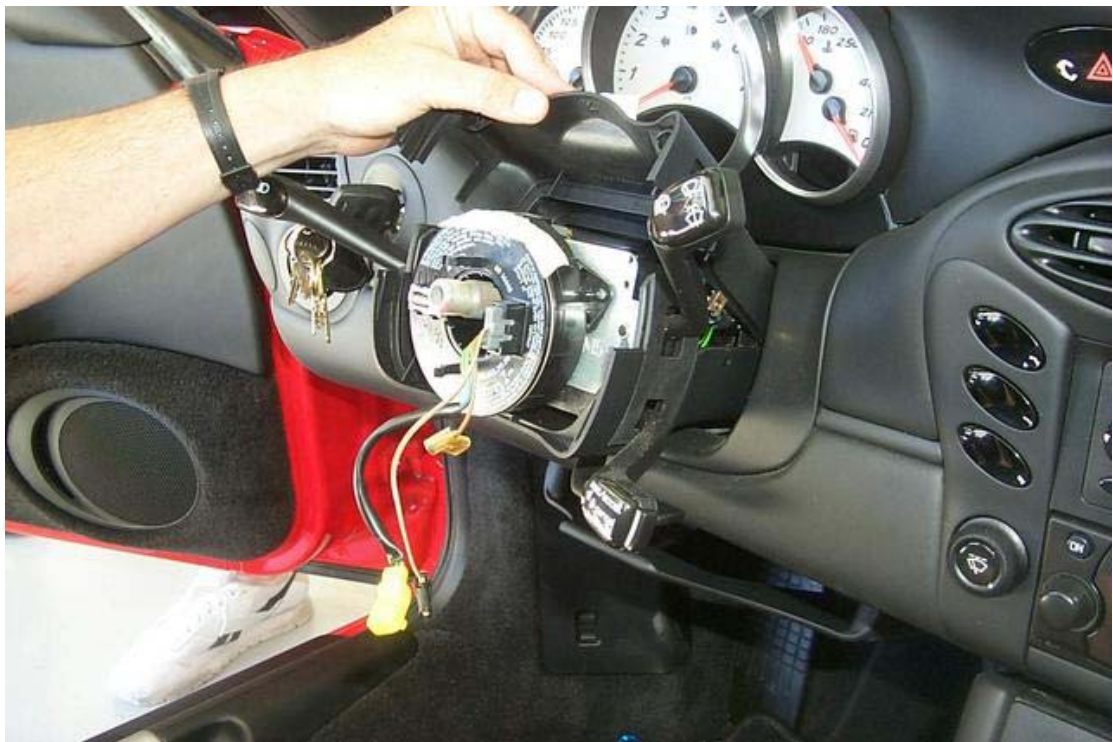
19 remove steering column upper housing – pay attention to how wires are routed inside!!
