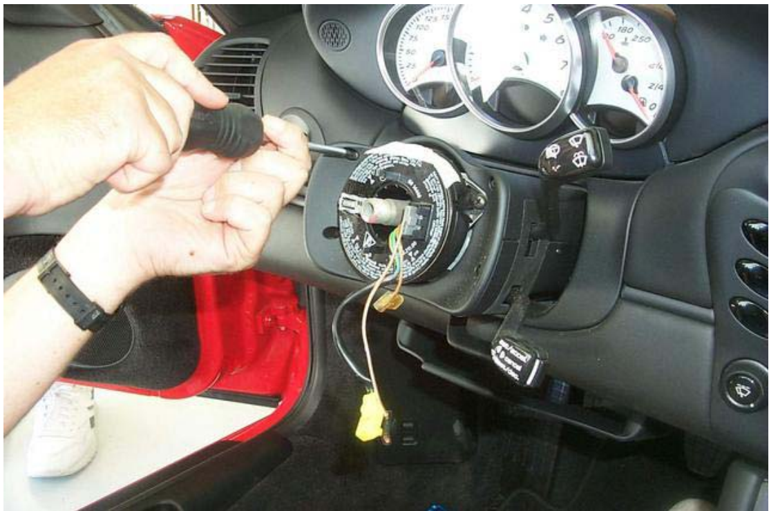
15 remove four Phillips screws holding steering wheel fascia piece on.
