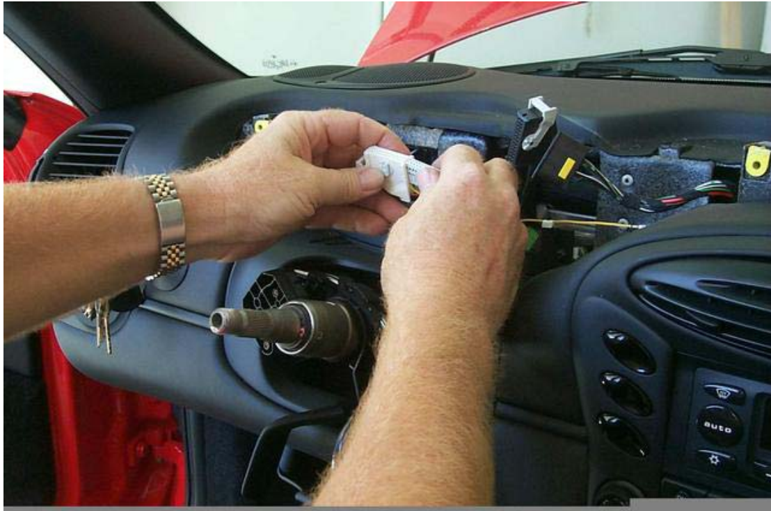
35 disassembling connector to install wiring harness connectors
