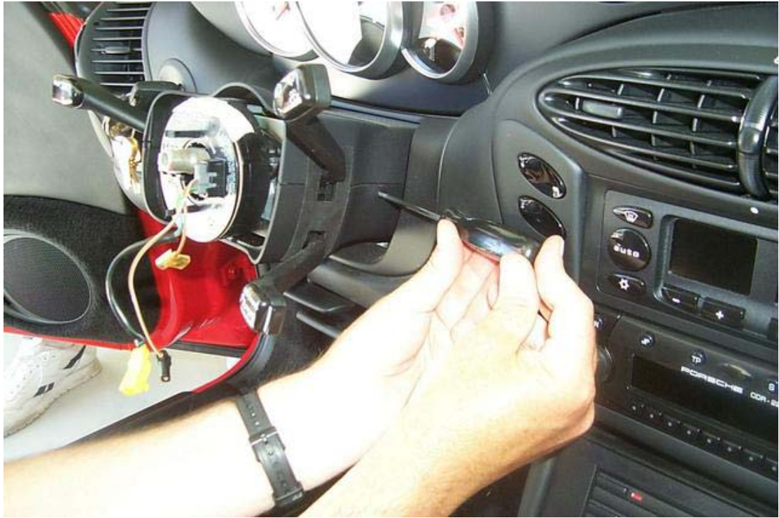
18 remove small torx (t-10) screws – may be Philips – one each side
