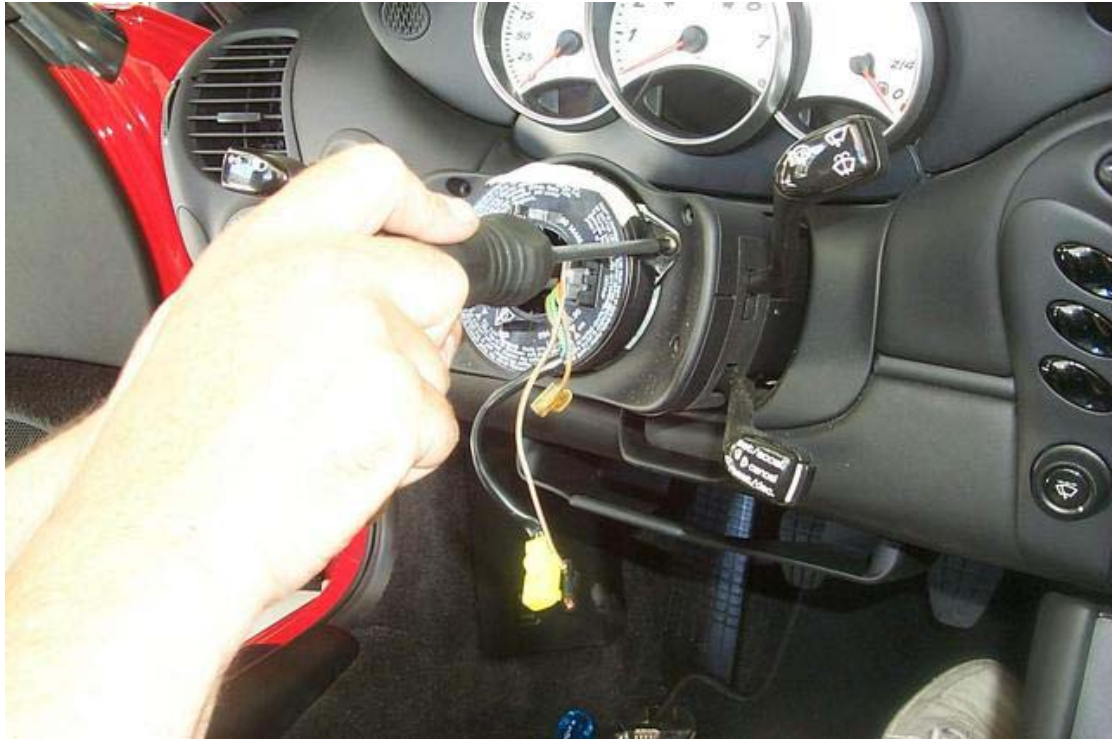
45 install philips screws holding air bag spring unit on (note 3-stalk assy pic used here)
