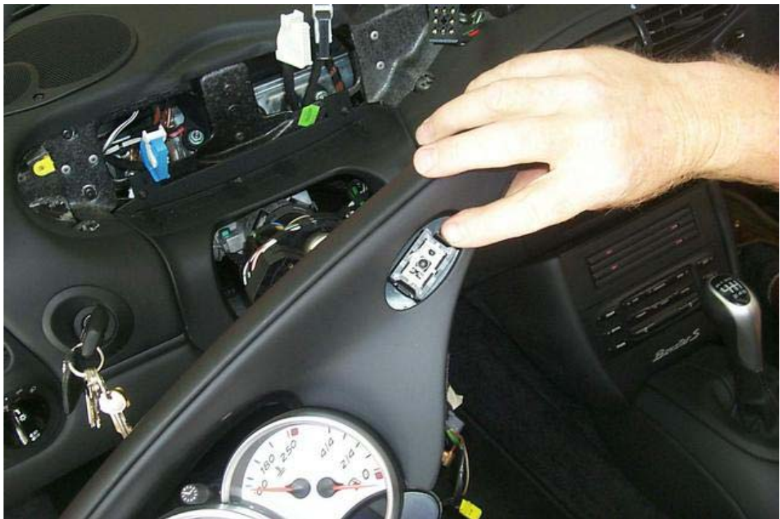
31 remove instrument pod. Screws are inside microphone on left and inside 4-way flashers or right – pull microphone & flasher button straight off to access screw
