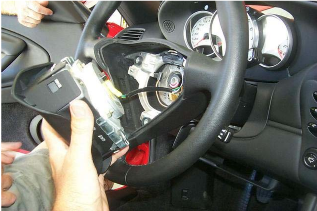
04 remove airbag unit, use thin flat tool to pry off airbag connector 02
